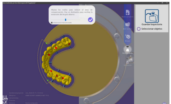
Fig. 12: The nesting of the suprastructure in MillBox CAM software.
