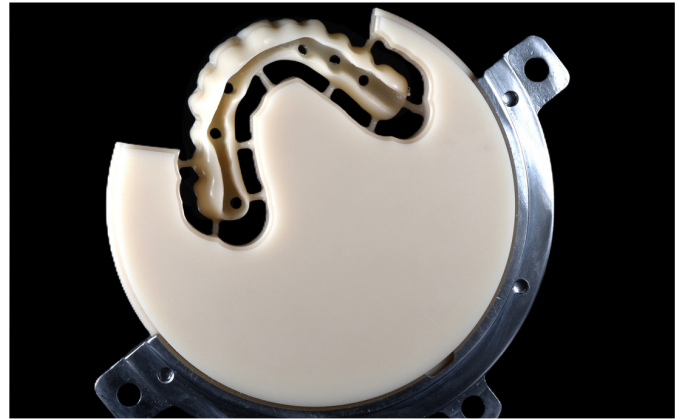
Fig. 14: The milling result of the suprastructure in the basal view.
