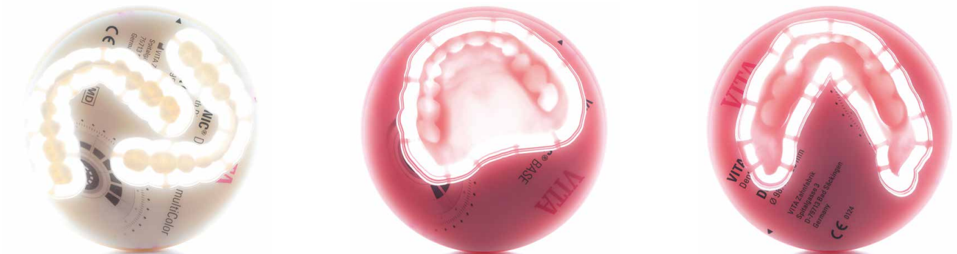
Fig. 3 to 5: The components of the full denture were subtractively manufactured using the milling blanks VITA VIONIC DENT DISC multiColor and VITA VIONIC BASE DISC HI.
